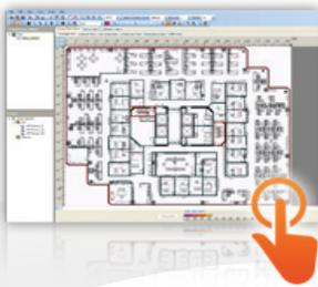
AirTight Planner supports both indoor and outdoor RF planning. You can import floor maps as AutoCAD files (DWG and DXF) or image files (JPEG, GIF, BMP).
